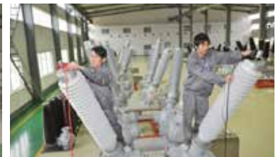
Circuit resistance measurement
