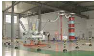
Voltage withstand routine test
