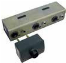
VDS HR and its removable luminous indicator
