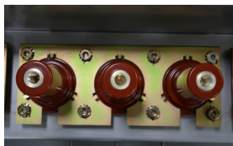
C / F / V : plug-in bushing NF EN 50181, with C type connection (I r : 630 A; Ø M16 mm)
